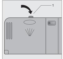
**2.** Fill the detergent dispenser with detergent. The markings indicate the dosing levels:
